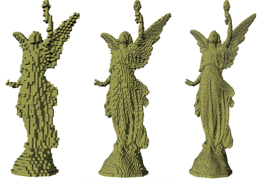
Figure 5: First-layer mesh of Lucy with different depths of the first-layer tree A . Quantization precision ( p value): 6, 7, 8 from left to right.
