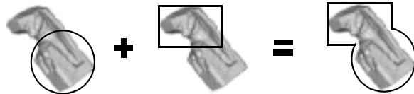
Figure 15: A hybrid structure obtained via the union of a sphere and an AABB
