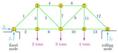
For the truss to be in static equilibrium, there must be no net force, horizontally or vertically, at any joint. Notice that each beam that is
