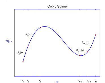
we want to construct a cubic spline S(x) to interpolate the table of values presumably of a function f(x). We assume that the points are ordered so that
