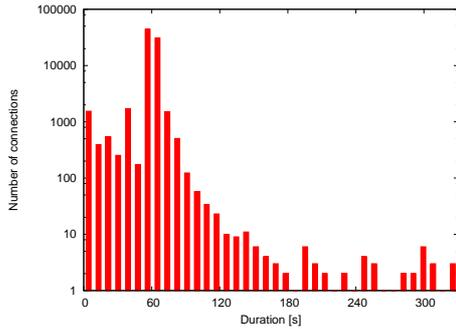
Fig. 4. Histogram of TCP connection durations
